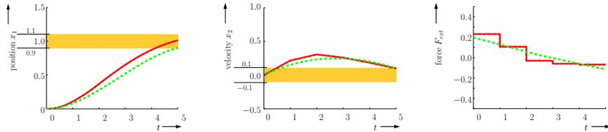
Figure 5: Approximate solution of the optimal control problem with state-dependent switchings. Solid lines: piecewise constant control, dashed lines: piecewise linear control.
