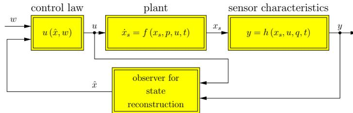
Figure 2: Observer-based closed-loop control of nonlinear dynamical systems.
