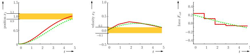
Figure 5: Approximate solution of the optimal control problem with state-dependent switchings. Solid lines: piecewise constant control, dashed lines: piecewise linear control.
