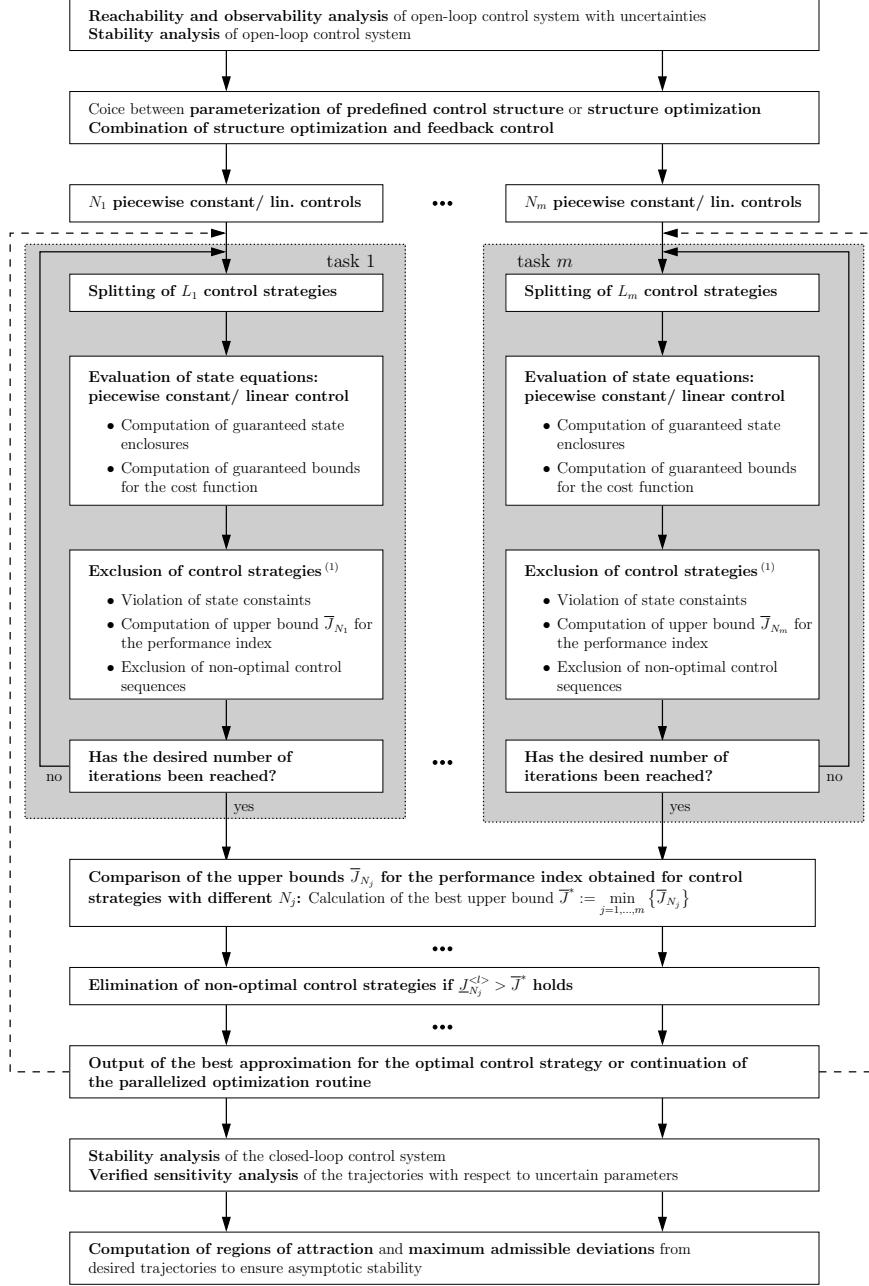
(1) Extension to robust trajectory planning by exclusion of inadmissible controls and inadmissible reference signals
